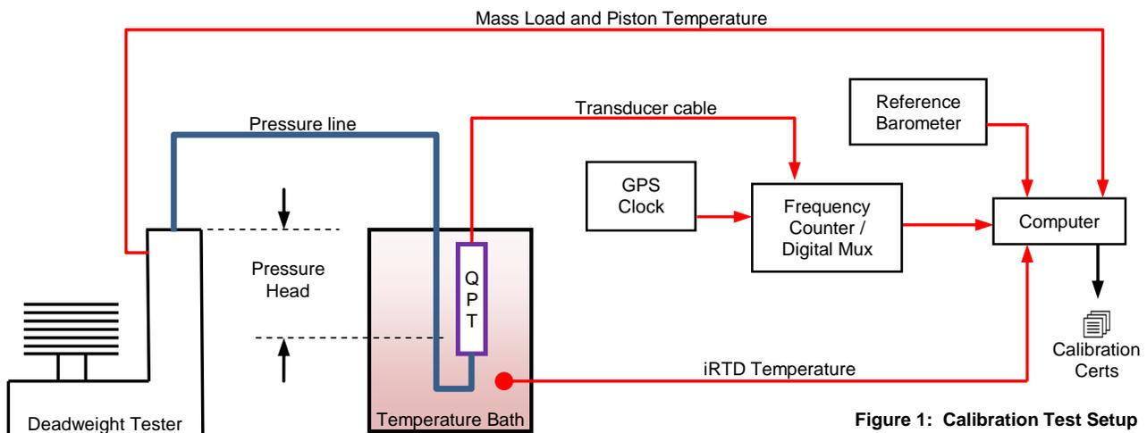
Figure 1: Calibration Test Setup
