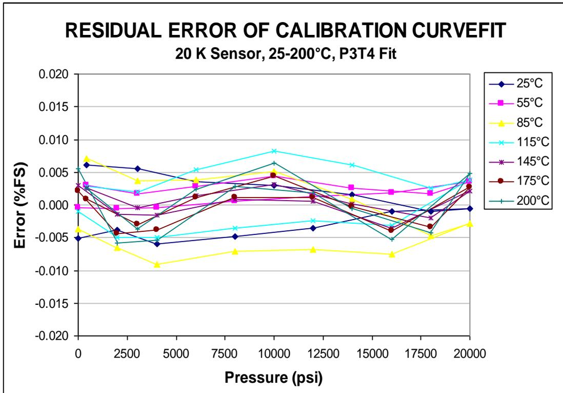
**Figure 2: Calibration curve typical of a Quartzdyne® Pressure Transducer**
