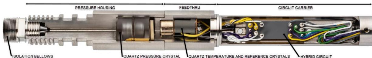
*Figure 1: Cross-Section of Typical Quartzdyne Pressure Transducer with Key Elements Identified*
