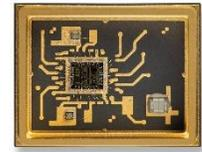
Figure 7: Next generation “analog” hybrid circuit. ASIC eliminates 23 additional parts.
