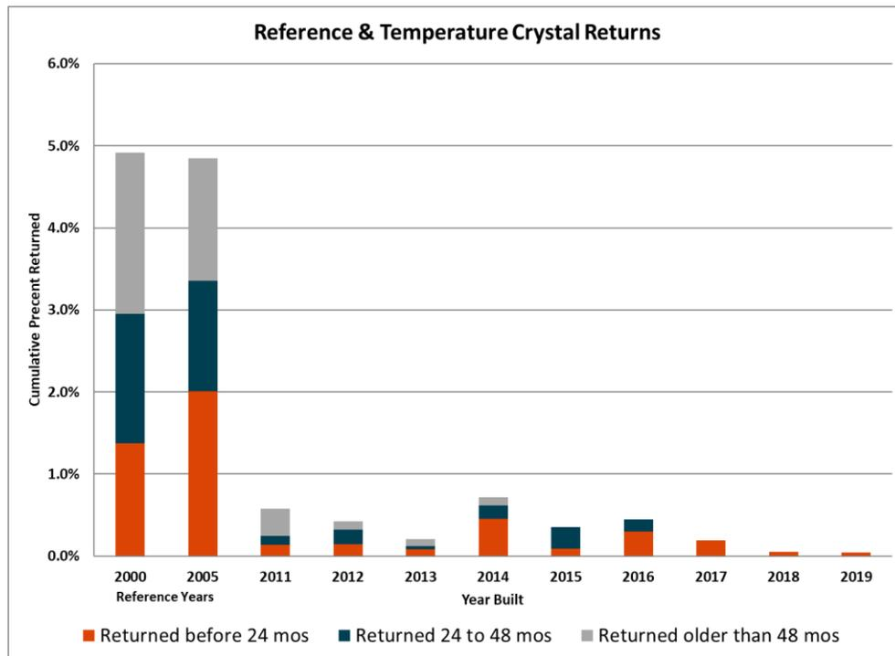
Figure 4: Reference and Temperature Crystal Reliability
